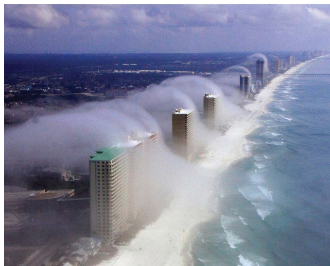
Figure 6: Flow displacement over high-rise buildings in Panama City Beach, United States. Wind is from the ocean. Source: Oke, T. R., Mills, G., Christen, A., & Voegt, J. A. (2017). Urban climates . Cambridge university press. (Photo Credit: J. R. Hott, Panhandle Helicopters; with permission).
